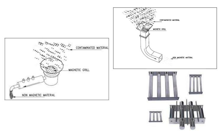
As the material flows through the grills, the iron particles are attracted by the magnets and they are trapped over the surface of the element. The trapped material has to be removed manually after removing magnetic grills from its location. In case of self cleaning grills the iron particles get trapped over the extra sleeve provided on the elements, they get released as soon as the elements are pushed out of the sleeves.
